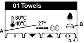
• When the moisture level detected by the dryer is equal to the level programmed, the dryer will enter the cooling stage and end of the cycle (see Example 1).
