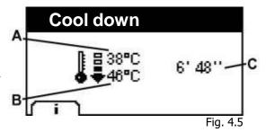
Once the cooling stage has ended, the machine informs the user of the end of the drying cycle acoustically and on screen.
