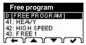
The option for using the manual program must be enabled in the OPTIONS menu from the System Tools menu. (Chapter 7).
