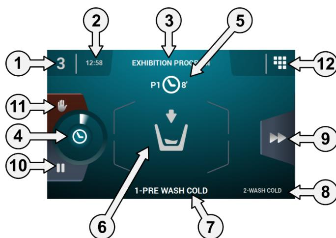
1. **Machine identifier:** Label identifying the machine.
