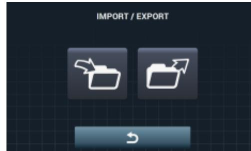
If IMPORT is selected, a screen is displayed to permit browsing through the USB. But only configuration files (with extension .cfg) can be selected.
