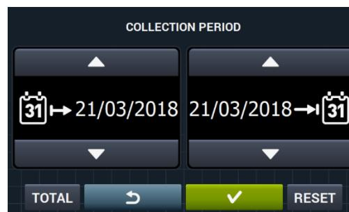
Press "TOTAL" to display the total values for the machine. If a date is entered, the statistics are only shown for this period. Press "Reset" to set all the values to 0, resetting the statistics.
