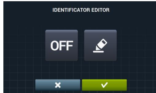
The machine identifier is enabled by pressing “OFF” followed by the edit button .
