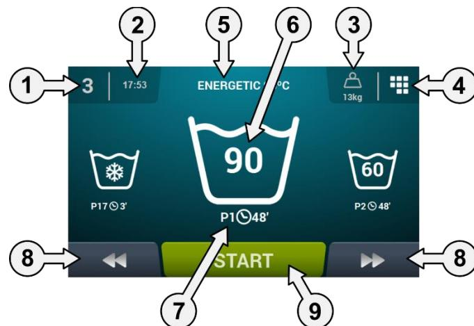
1. **Machine identifier:** Label identifying the machine.
