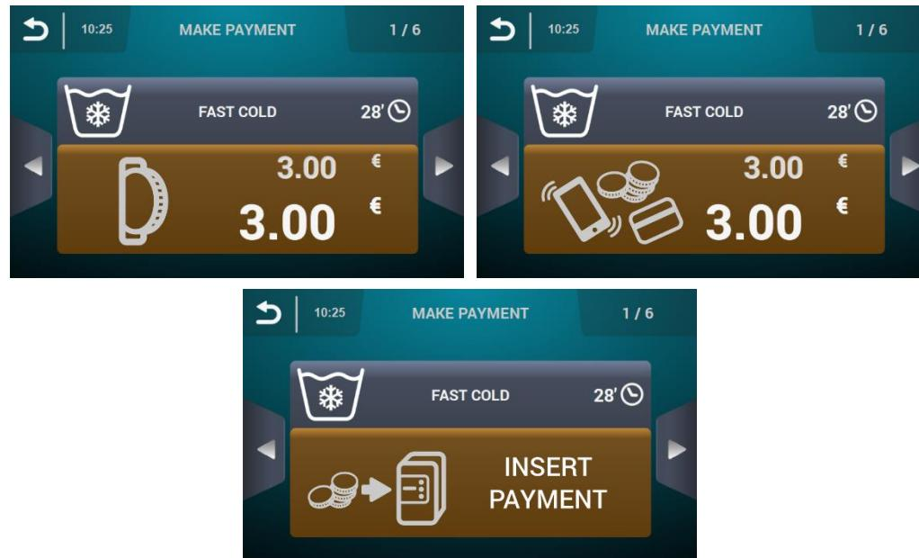
The button is displayed in brown until the amount indicated in the program has been inserted in the machine.
