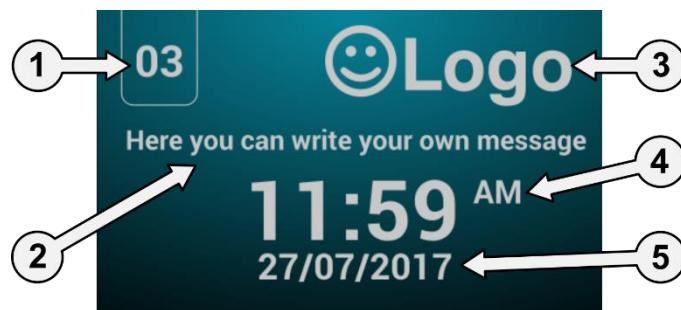
1. **Machine identifier:** Label identifying the machine (if enabled).
