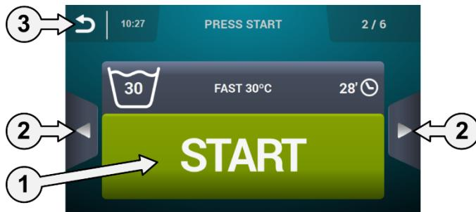
1. **Start Button:** When the program amount has been inserted, a large "Start" button is displayed in green.
