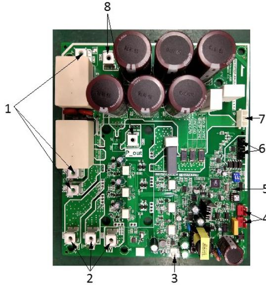
Table 5-3.1: Compressor inverter module PCB ports
