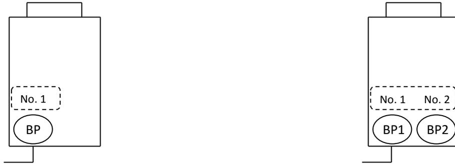
Figure 3-4.2: Compressor priority and rotation – two outdoor units
