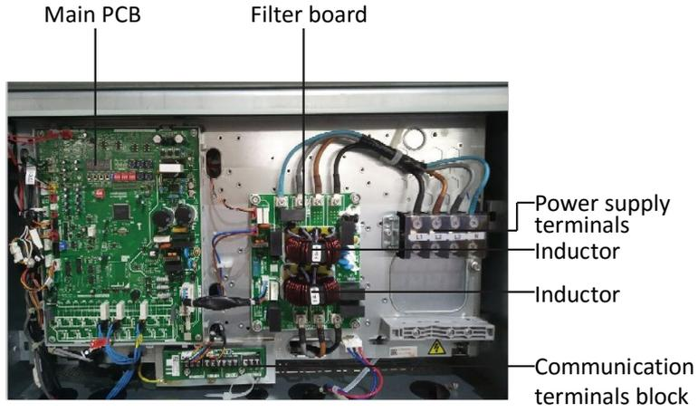
Figure 5-1.4: 18-30HP bottom layer of electric control box
