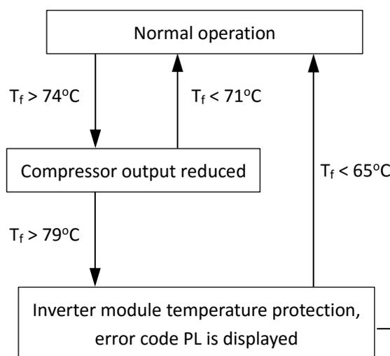
When PL protection occurs 3 times in 100 minutes, the C7 error is displayed. When a C7 error occurs, a manual system restart is required before the system can resume operation.
