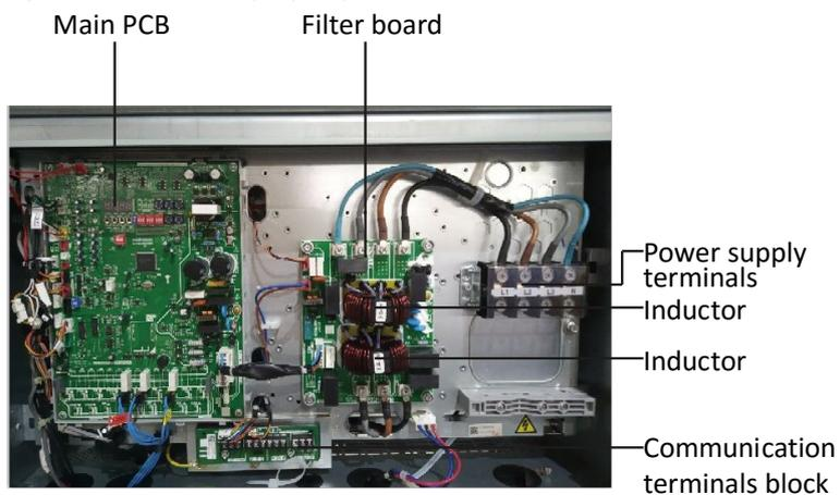
Figure 5-1.2: 8-16HP bottom layer of electric control box
