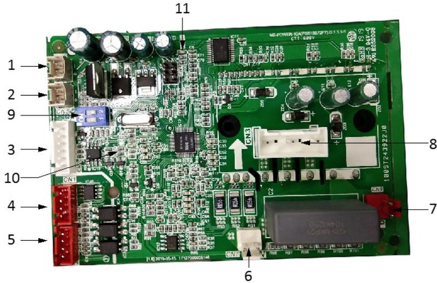
Table 5-4.1: Fan module PCB ports
