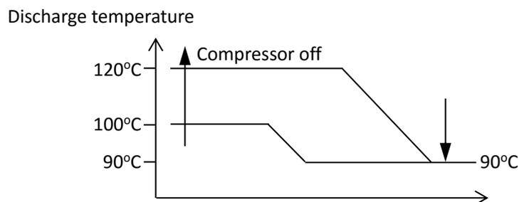
When the discharge temperature rises above 120°C the system displays P4 protection and all units stop running. When P4 protection occurs 3 times in 100 minutes, the H6 error is displayed. When an H6 error occurs, a manual system restart is required before the system can resume operation.
