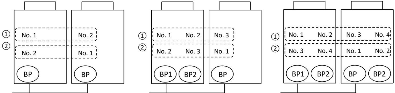
Figure 3-4.3: Compressor priority and rotation – three outdoor units
